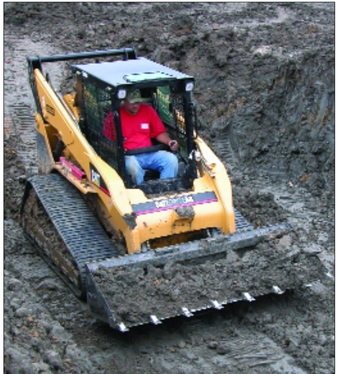
Soft underfooting is no problem with a multi terrain loader, working at the company's site on the east edge of Cedar Rapids, Iowa.
